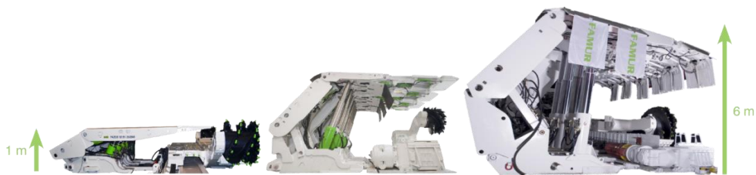
Roof supports and shearers made by FAMUR Group
