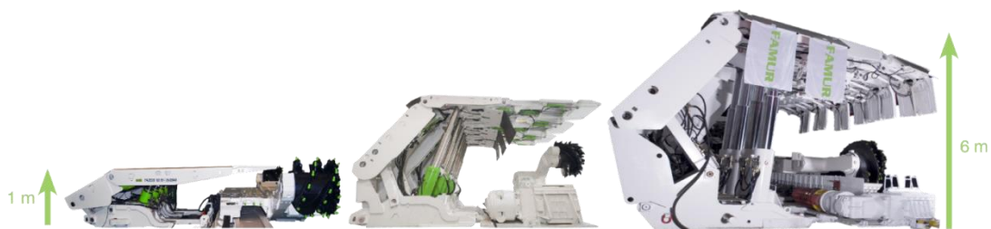
Roof supports and shearer loaders
